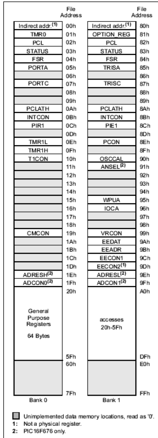
FIGURE 2-2: DATA MEMORY MAP OF THE PIC16F630/676
