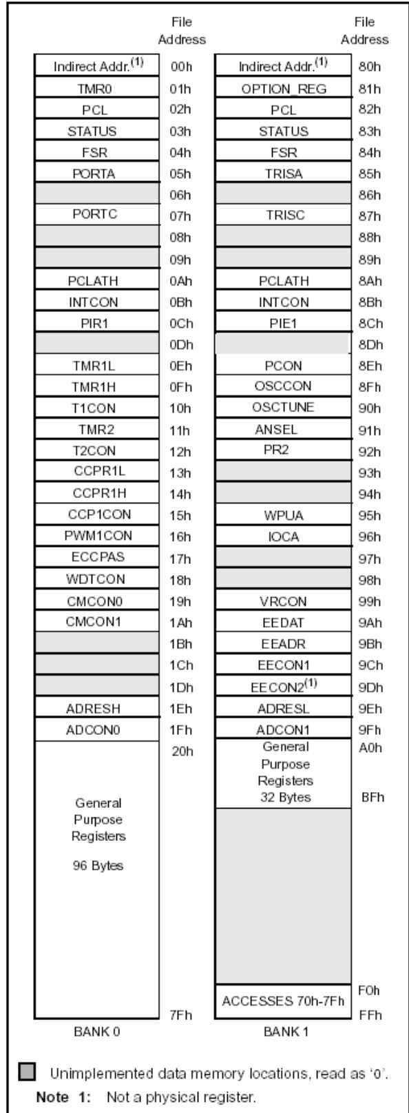
FIGURE 2-2: DATA MEMORY MAP OF THE PIC16F684
