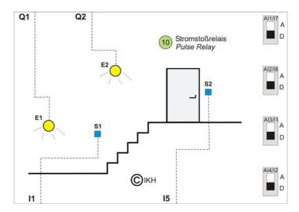
A pulse relay circuit is used to switch lamps E1+E2 on or off from two different locations with S1 or S2.
